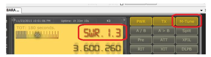
If the SWR meter indicates a SWR greater than 2:1, do not transmit at that frequency. Operating with a high SWR can damage the radio.
