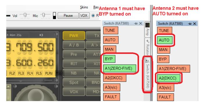
Either antenna is tuned by clicking the **M-Tune** button, which will cause the radio to transmit a low powered CW signal to force the appropriate tuner to tune the antenna for the new frequency. When the tuning cycle is complete, or 30 seconds has elapsed, the **M-Tune** button will turn off the tuning signal. When you click on **M-Tune**, wait for it to finish before clicking any other controls.
